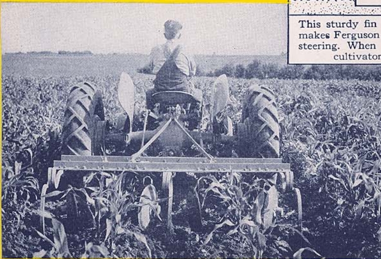
L-KO Listed Crop Cultivator Discs are reversible so dirt can be thrown toward or away from plants, depending on stage of growth.
